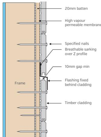
Minimum clearance of cladding above final ground levels and finishing below bottom plate
